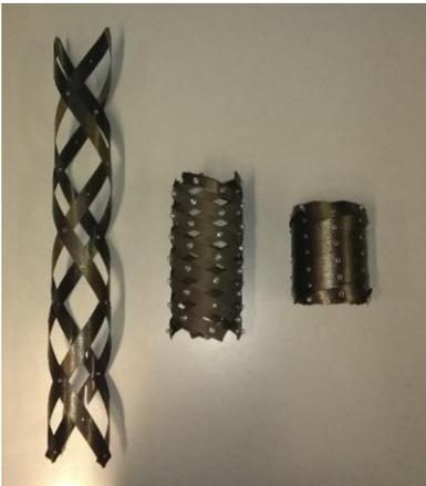
Figure 1: Three lattices with different stability point locations
