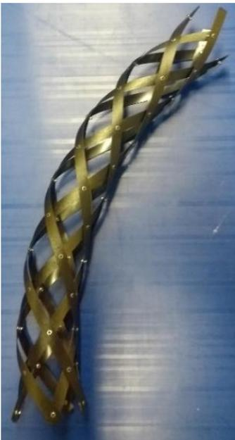
Figure 2 Morphing lattice with a curved deployment path
