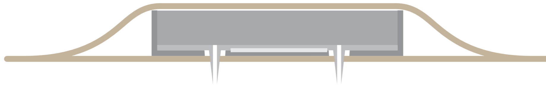
The needle bed would perforate the bottom layer of material and into the skin allowing for the blood sample to be taken
