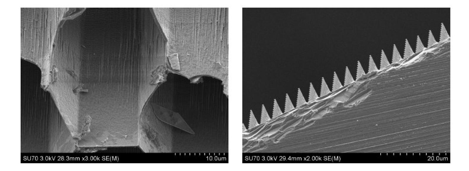
Figure 3. SEM images of lithography etched devices in a (left) honeycomb pattern and (right) pillar pattern. The picture on the left shows the defects in the walls with the inset revealing the overall structure. The picture on the right shows the well aligned pillars tilted at 15 degrees. Material is courtesy of Dr Ryan Enright (Stokes).
