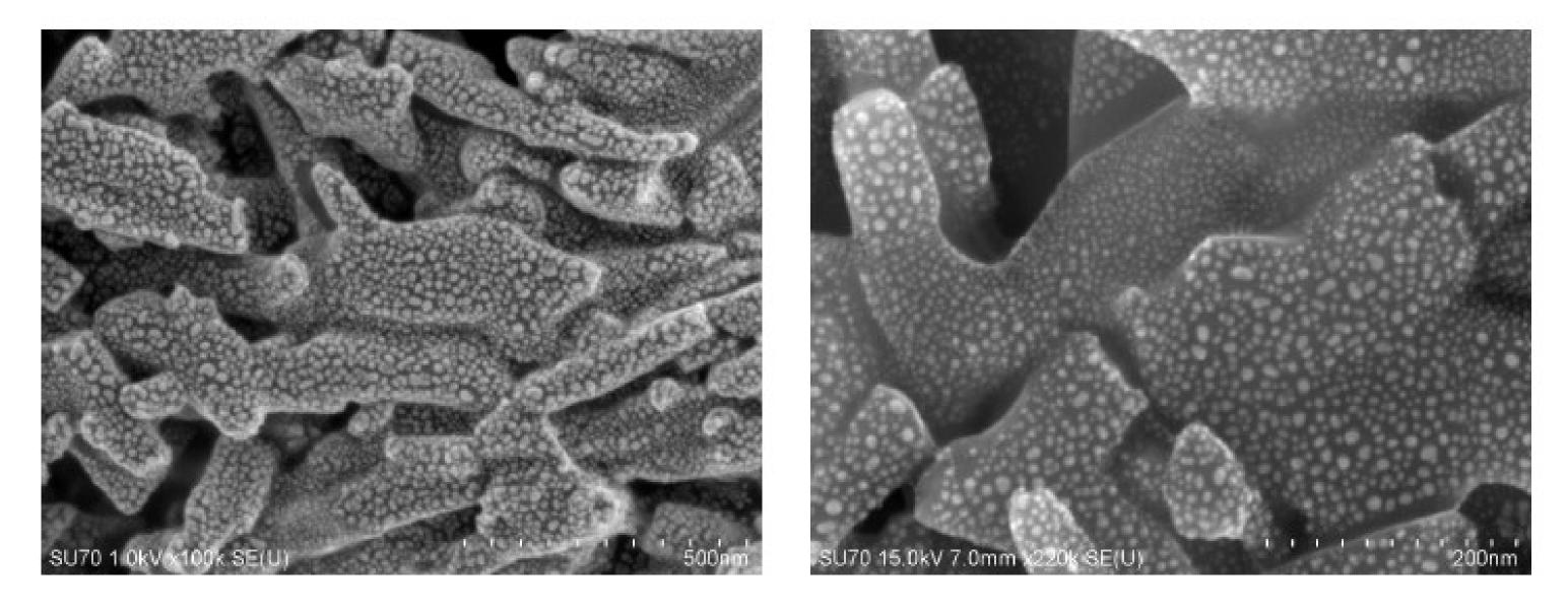
Figure 1. Images of gold islands on conducting film using the upper SE detector at (left) 1kV and (right) 15kV. The resolution remains similar indicating that using the lower voltages for uncoated beam sensitive materials can be done without loss in resolution
