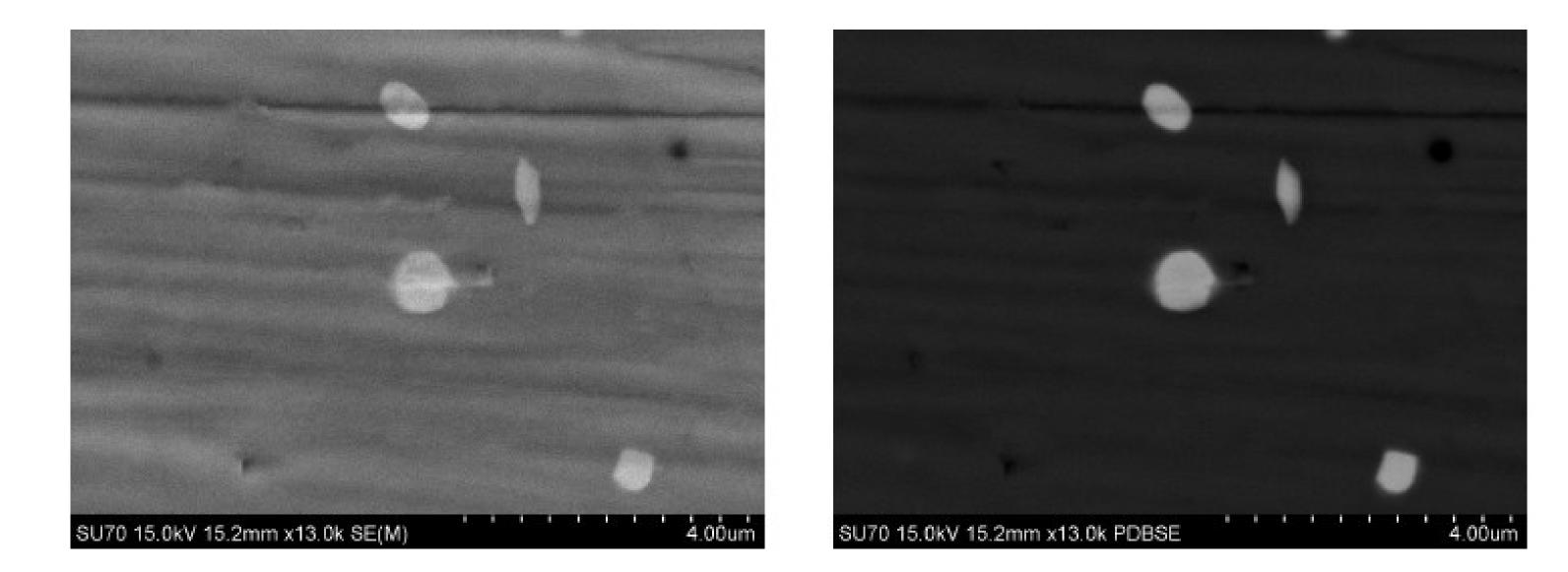
Figure 2. SEM images using (left) SE detectors and (right) BSE detector on a transition metal containing a lanthanide metal. The lanthanide is heavier, and therefore the contrast is stronger in BSE mode. Material is courtesy of Dr Tofail Syed
