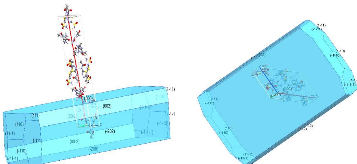
**Figure 2: BFDH representation of an equimolar binary acetazolamide-theophylline co-crystal (C2/c, A:T 1:1). The binary co-crystal is characterized as a monoclinic system – with respect to crystal symmetry, it is centrosymmetric.**
