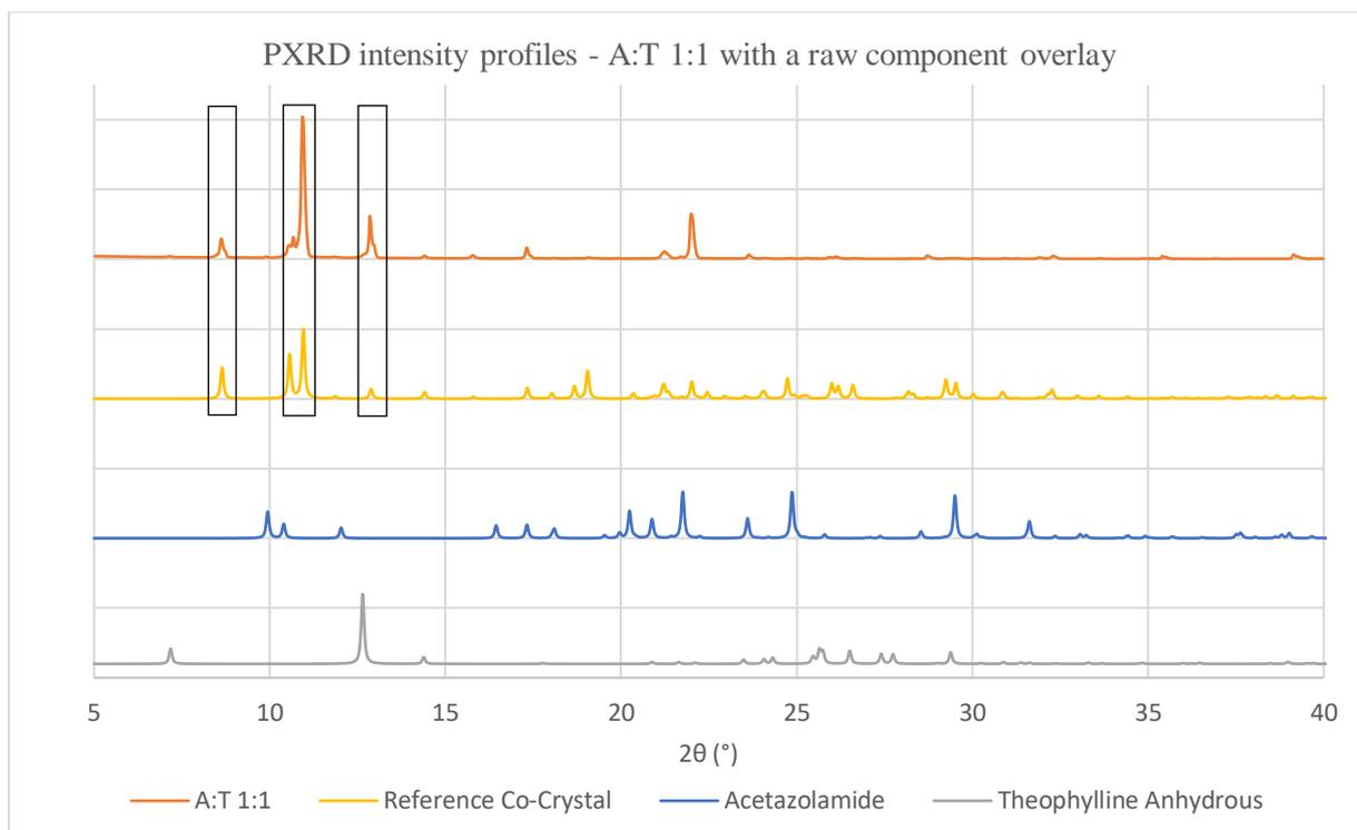
Evidence of binary co-crystal formation via PXRD gave justification for the use of liquid-assisted grinding in other co-crystal syntheses. This method was therefore extended to the synthesis of a multicomponent co-crystal of acetazolamide (ACZ), theophylline anhydrous (THP) and microcrystalline cellulose (MCC). FTIR analysis provided compelling evidence of multi-component co-crystal formation, specifically the binding of MCC to the binary co-crystal:
