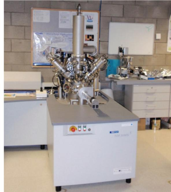
A self-adjusting charge compensation system using a low energy electron flood gun synchronized with ion gun pulsing to neutralize the positive charge after each ion pulse. A 30 keV, three-lens BiMn cluster ion gun. This cluster Liquid Metal ion Gun (LMIG) is ideally suited for high lateral resolution microanalysis and imaging as well as high mass resolution surface spectroscopy.
